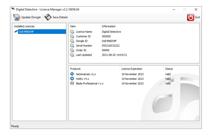
With the USB dongle inserted into a free USB slot, run the Licence Manager software. It should show the active dongle in the left hand pane. Click the **Save Details** button to save information relating to this dongle.
